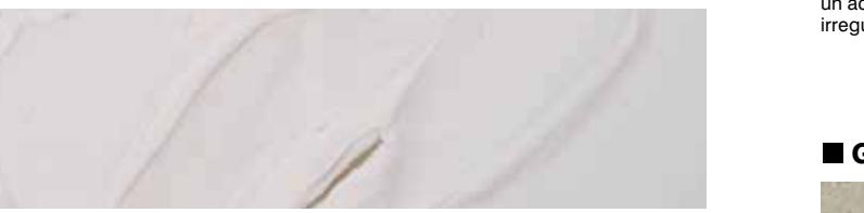
**EN** Finely textured smooth white marble paste. Once dry, surface can be carved and sanded. The product can be used as mortar and filler on constructions and joints.
